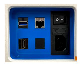
• System Power - The main system power components consist of the power switch and power input.
