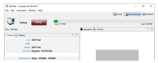
To view the log when the test is done, select **Instrument**, click **Properties** and click **Logs**. Select the test log you would like to view and click **View**.
