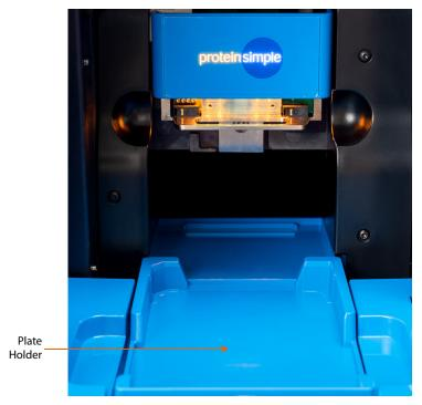
Sample plates should be inserted into the plate holder so that the A1 well position is aligned with the upper left corner of the tray.
